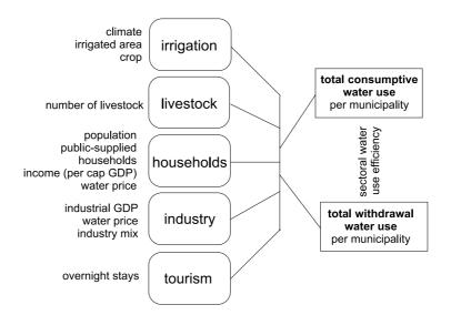
Figure 1. Overview of the regional water use model, showing the driving forces of the water use sectors irrigation, livestock, households, industry and tourism.
