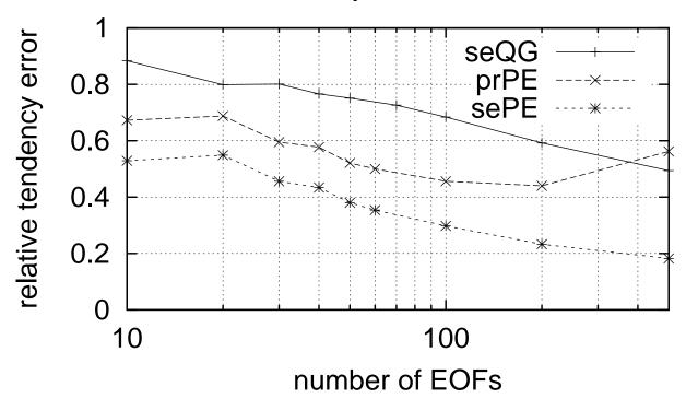
Figure 2: The relative error in the prediction of GCM tendencies (in a data set with seasonal cycle) by the semi-empirical and projected reduced models with primitive equation core, depending on the number of EOFs the model is based on. Also shown are the corresponding results from Achatz and Branstator (1999) for the prediction of tendencies in a perpetual-january data set of a GCM by a semi-empirical reduced model with a quasigeostrophic two-layer model core.
