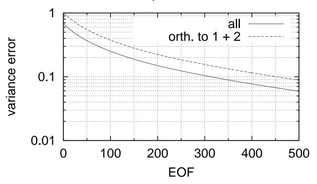
**Figure 1**: The relative variance not explained by using a given number of global EOFs, for the total variance and the variance orthogonal to the two leading patterns. EOFs 1 and 2 describe most of the seasonal cycle.
